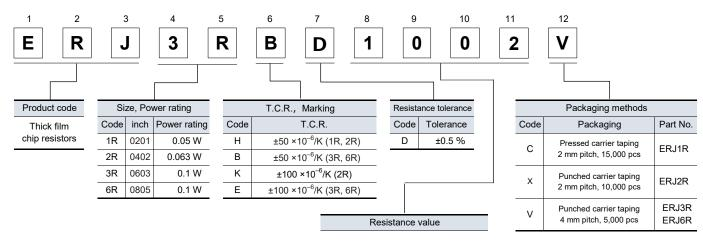
The first three digits are significant figures of resistance and the last one denotes number of zeros following. Example :  $1002 \rightarrow 10 \text{ K}\Omega$
